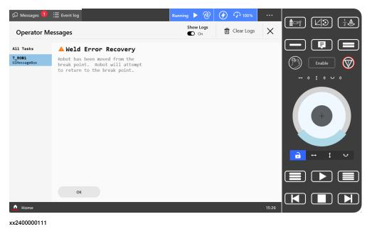
Tapping OK moves the robot to the recovery set point.
